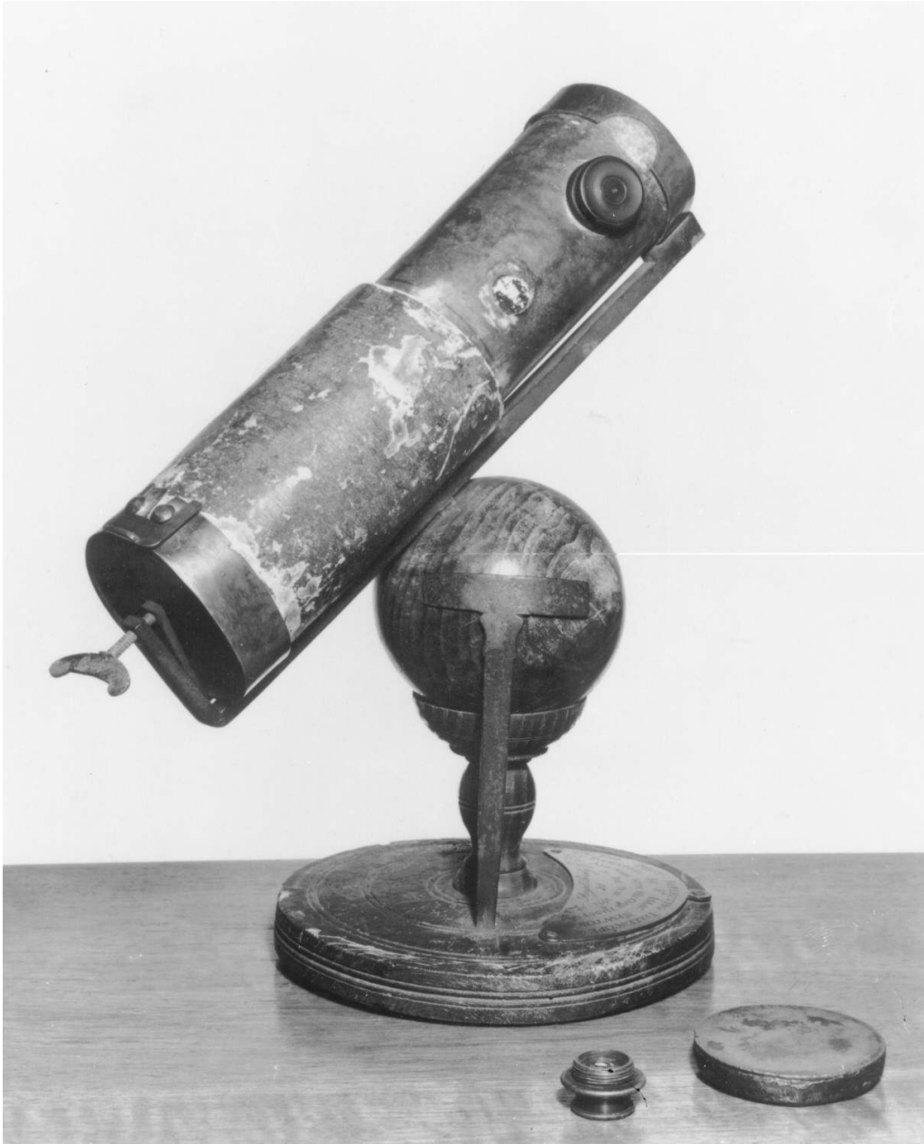
Figure 1.2 The reflecting telescope that Sir Isaac Newton built and gave to the Royal Society in 1671. By kind permission of the Royal Society. © The Royal Society.
